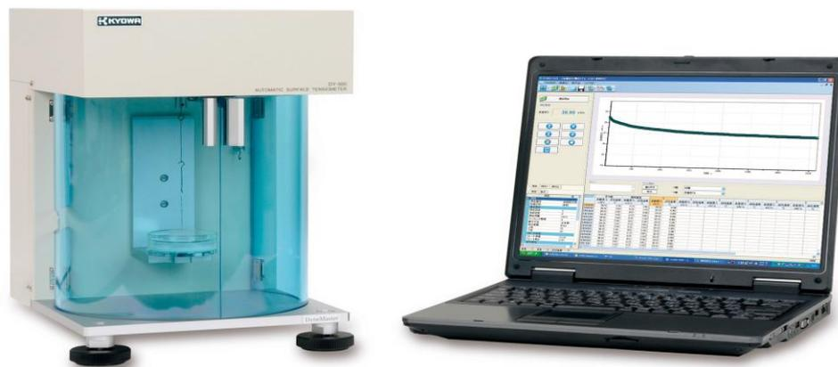
With Kyowa's long-standing experience and great engineering expertise, the only handicap of a stand-alone Tensiometer – namely, the volume of sample needed, has also been overcome. This simple yet ingenious accessory is the Teflon Lab Dish which is very narrow and it takes a maximum of only upto 2ml volume and wide so that it wets the entire breadth of the Wilhelmy plate.
